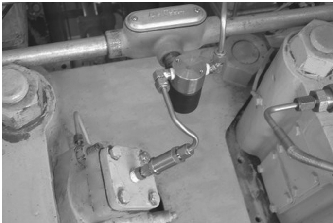
Pneumatic air distributor with pilot-actuated air-in-head valve
