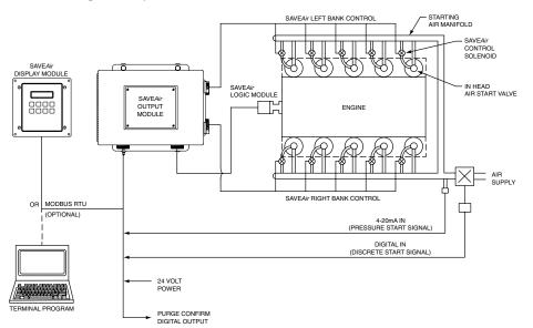
spots" — and to drastically reduce the amount of starting air required. More reliable remote starting, improved operator safety (no mechanical barring), reduced air consumption, and more efficient compressor station operation are just a few of the benefits of SaveAir<sup>™</sup> operation.
