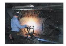
Thermex<sup>®</sup>-Thermal Spraying-Exline selects from hundreds of metallic and nonmetallic coating options and five thermal sprav processes to achieve the surface characteristics you require, such as abrasion resistance, lubricant retention, and corrosion protection.
